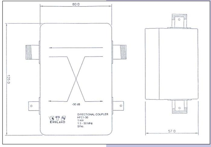
\*The coupler is effective over a very much wider frequency range with a small degradation in performance. Calibration charts can be supplied for those out of band frequencies, where for example, measurement of harmonics is desired.
