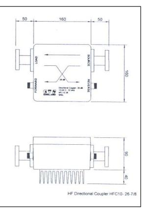
\*The coupler is effective over a very much wider frequency range with a small degradation in performance. Calibration charts can be supplied for those out of band frequencies, where for example, measurement of harmonics is desired.
