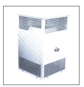
The RL100-5 is a 50 ohm unbalanced resistive load designed specifically for the HF frequency range 1.5 - 32MHz. The load is convection cooled, requires no AC power and is suitable for outdoor unprotected operation. Typical applications include use as a transmitter load, hybrid balancing load and antenna common mode load.
