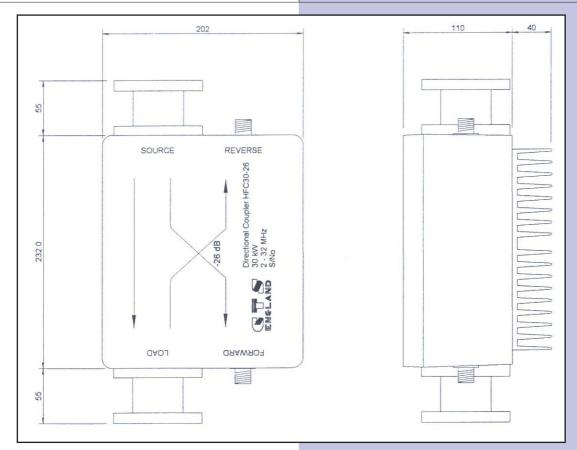
\*The coupler is effective over a very much wider frequency range with a small degradation in performance. Calibration charts can be supplied for those out of band frequencies, where for example, measurement of harmonics is desired.
